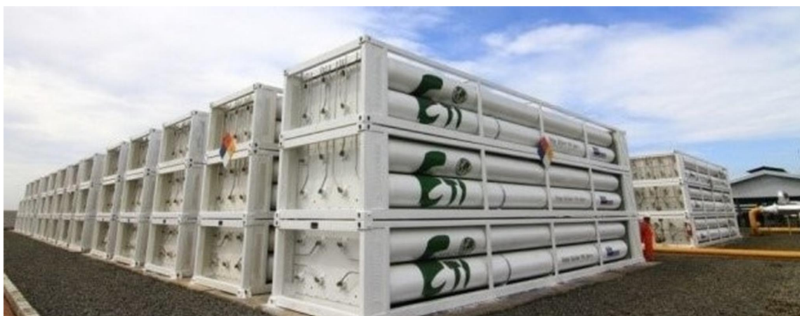
Figure 3.3.3. CNG cylinders, length 40 ft (12.192 m), 8-cylinder skid (CIMC Enric, China)
